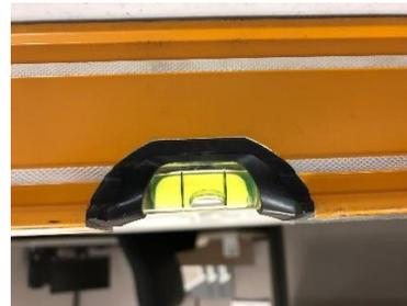
In this picture, the bubble is too close to the line and will cause walls to be out of plumb by up to 1+” or windows to not close properly.
